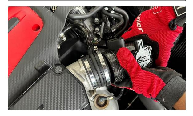
STEP 8: Tighten the hose clamp to secure the inlet tube. DO NOT OVERTIGHTEN.
