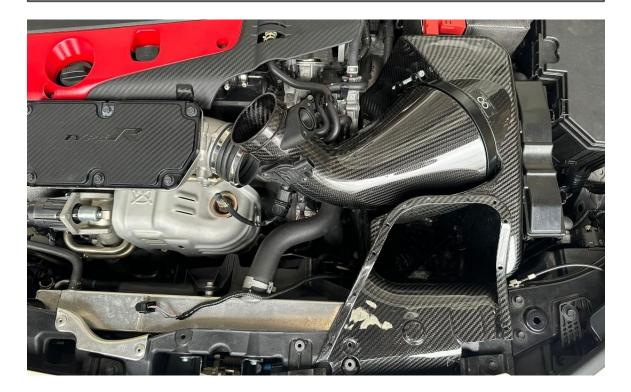
**STEP 7:** Rotate the inlet tube clockwise and push it into the EPDM coupler.
