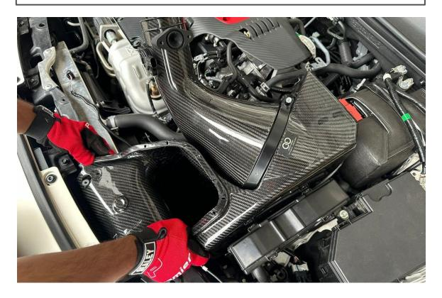
**STEP 6:** Push the airbox down to secure the grommet into the stud. Once in position, the front bolt hole should line up.
