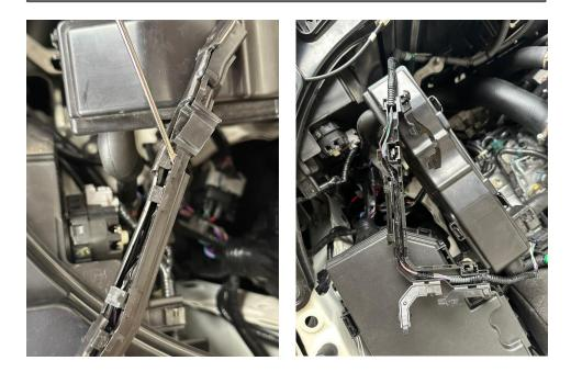
**STEP 15:** Use the provided split loom to cover the exposed wiring, cutting any excess.
