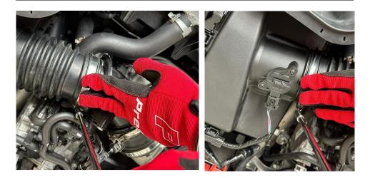
**STEP 7:** Squeeze the corrugated tube to remove.
