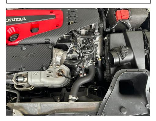
**STEP 11:** Remove the OEM rubber coupler and plastic breather pipe.
