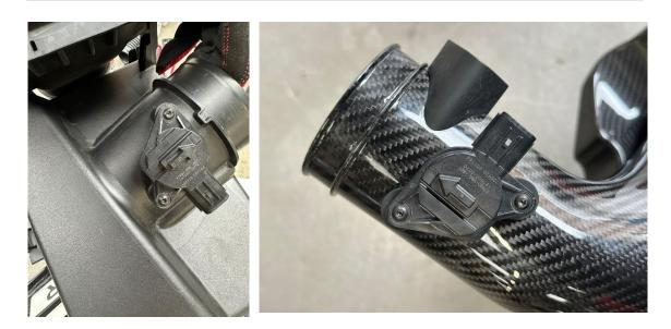
**STEP 2:** Assemble the airbox in the order shown. Tighten the v-band clamp enough so that the tube is secure but can rotate.
