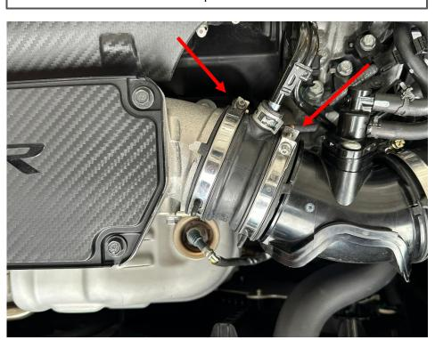
**STEP 10:** Remove the two Torx screws securing the breather.
