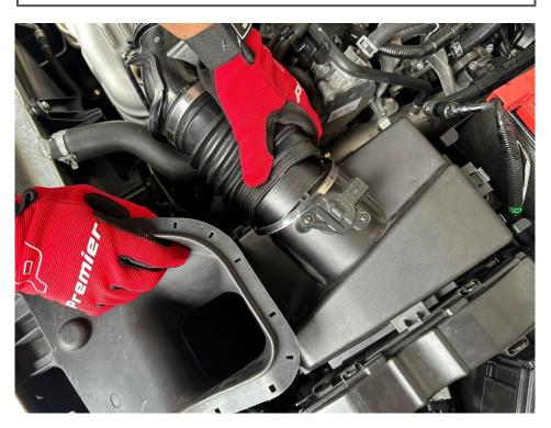
**STEP 8:** Use plyers to remove the spring hose clamp.
