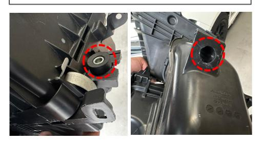
**STEP 14:** Use a flat head screwdriver to pry open the plastic shroud protecting the MAF wiring
