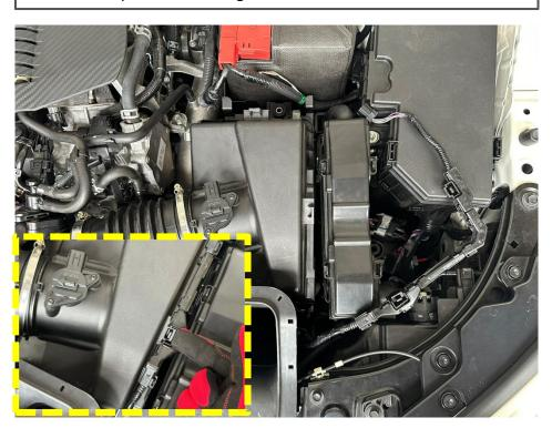
**STEP 6:** Undo the hose clamps securing the corrugated rubber tube.
