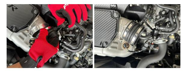
**STEP 5:** Rotate the inlet tube upward. Tilt the assembly forward and slide the front feed in.
