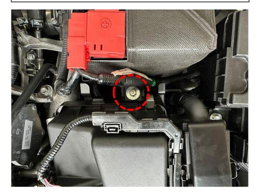
**STEP 3:** Remove the front lower airbox bolt.
