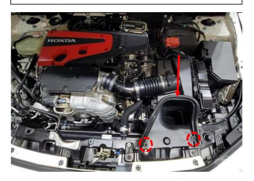
**STEP 2:** Remove the bolt at the rear of the airbox.
