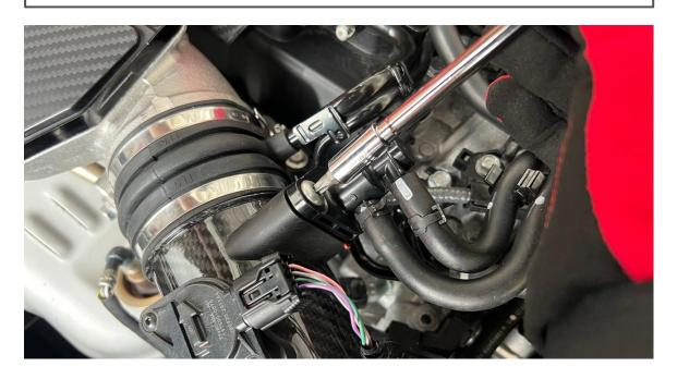
**STEP 12:** Use the OEM bolts to secure the front and rear of the airbox. **DO NOT** tighten the screws, thread them in and leave them as shown in the pictures.
