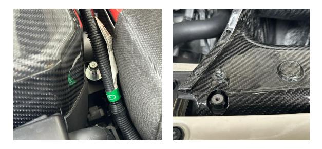
**STEP 15:** Install the weather stripping, pushing the plastic pins into their respective holes.
